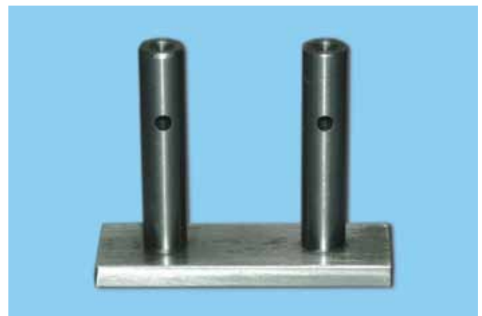
2 Metal jig (37 mm (L) × 14 mm (W) × 3 mm (H)) with V-shaped crater on top of vertical beams for measuring references and with setting pin holes to stop guides at same vertical position.
