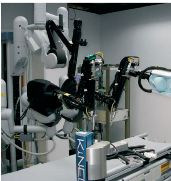
Figure 5. Tool autoloader subsystem (TAS) mounted on a da Vinci arm
