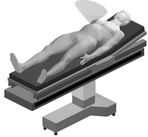
Fig. 4. Workspace in MIS: an elliptical cone with vertex angles of 60^\circ and 90^\circ represents the workspace such that the endoscopic tool can reach any organ in the abdomen. The ports are placed such that the end-effector of the tools can access the target anatomy. In this illustration, the port is located at the center of the abdomen with the cone at 90^\circ elevation.
