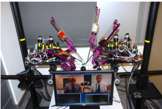
Figure 2 Two surgeons collaboratively teleoperate the RAVEN IV robot system located 900 miles away
