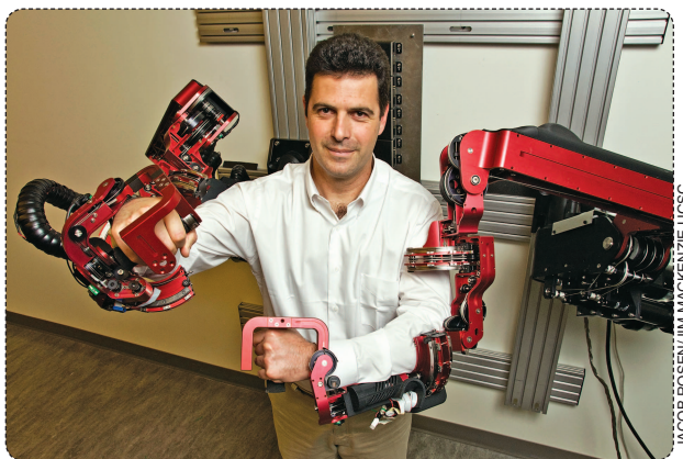
FIGURE 5 Prof. Jacob Rosen wearing the two-arm exoskeleton with seven degrees of freedom each. The system allows the user to reach 95% of the natural workspace of the human arm and provides assistance and guidance with forces that are similar to the forces produced by the muscles of a healthy individual. The system has applications in haptics (providing force feedback in virtual reality), teleoperation (controlling a robotic system from a distance). It is currently tested in the context of stroke rehabilitation utilizing a bilateral mirror-image mode of operation.
