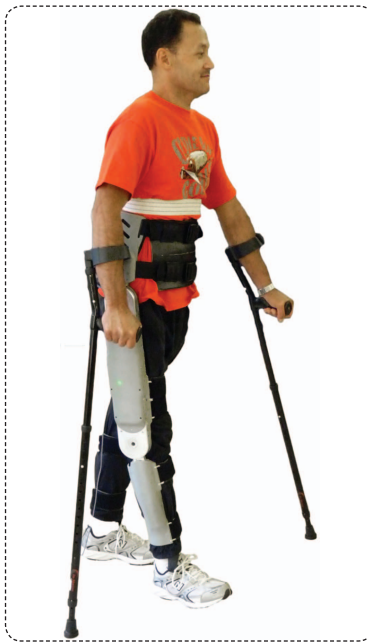
FIGURE 3 With the Vanderbilt exoskeleton, users can sit, stand, walk, and both ascend and descend stairs and slopes. (Photo courtesy of Ryan Farris and Hugo Quintero, Center for Intelligent Mechatronics at Vanderbilt.)
