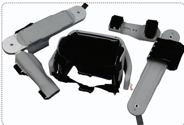
FIGURE 4 The Vanderbilt exoskeleton is a three-piece, modular device that quickly—and without tools—snaps on and off. (Photo courtesy of Ryan Farris and Hugo Quintero, Center for Intelligent Mechatronics at Vanderbilt.)
