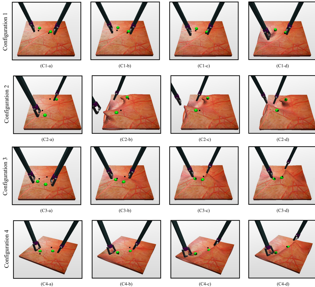
Fig. 3. Example successful policies. Four configurations (C1-C4) are displayed for representative progressing actions during testing episodes from (a) initialization to (d) task completion . Each configuration represents a different set of initial TTPs, IDPs, and TGP. Additionally, in (C4), the camera configuration is changed. In order to maintain simulation stability, it was necessary to manipulate TGPs via simulated springs with low stiffness connected to the graspers. As such, small gaps between graspers and the tissue are observable for large deformations.
