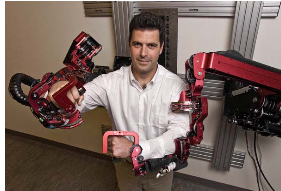
Fig. 1. The 7 DOF upper limb exoskeleton (EXO-UL7)
