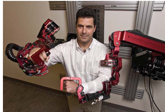
Fig. 1. The 7 DOF upper limb exoskeleton (EXO-UL7)
