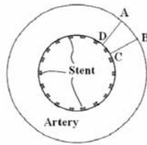
Fig. 2 - Artery and stent cross section at the middle of stent's beam
