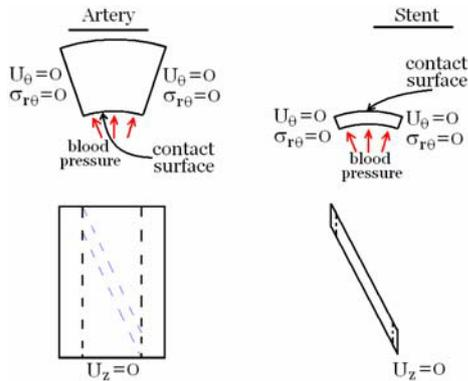
Fig. 5 - Boundary conditions as defined in the three dimensional model.
