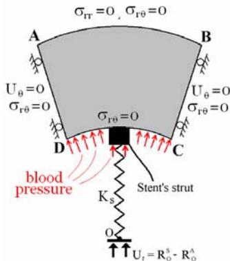
Fig. 3 - Two dimensional plane problem for a stent being inserted into an artery with the appropriate boundary conditions
