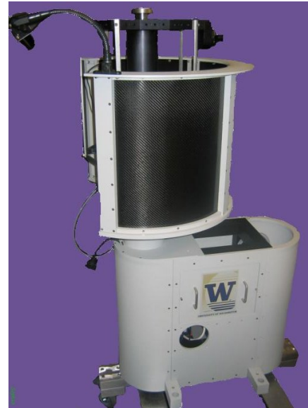
Fig. 3. Photo of completed Tool Rack Subsystem during testing. Graspers are not mounted onto the carousel in this photo. Video camera, mounted on a locking positioning stalk, is added to the frame to allow video monitoring of the tool exchange. Calibration fixture is visible pointing away from the tool presentation position (upper right).
