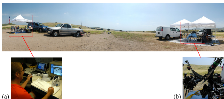
Figure 1. The surgical robotic system deployment in Simi Valley, CA. (a) The surgical Console (Master) (b) The surgical robot (slave)
