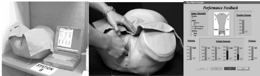
Figure 1. The Complete E-Pelvis Simulator, a Simulated Pelvic Exam, and the Graphical User Interface.
