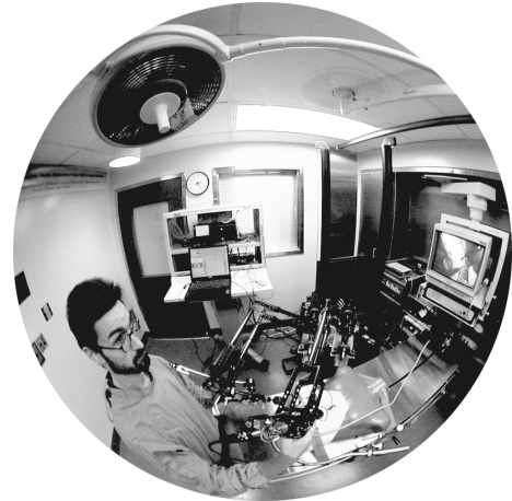
Figure 1: The BlueDRAGON system integrated into a minimally invasive surgery operating room
