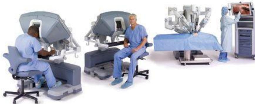
Figure 10: The da Vinci Si by Intuitive Surgical Inc. (a) Surgeon-side two surgical console (b) Patient-side subsystem
