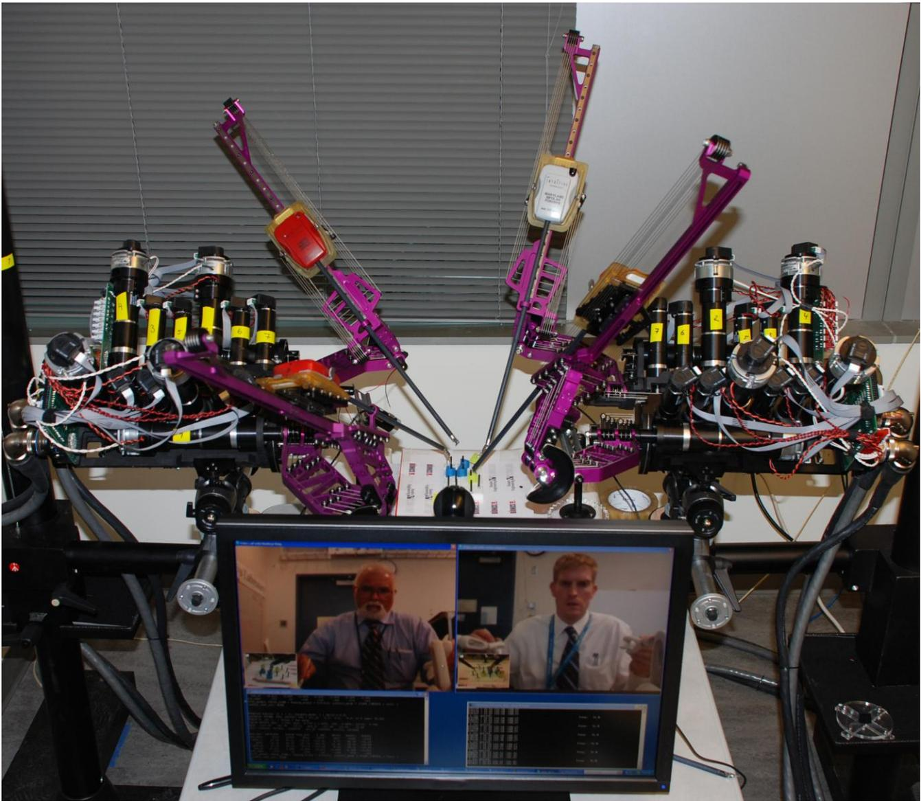
Figure 17: Raven II – A research platform for studying surgical robotics. The image depicts a teleportation experiment in which two surgeons located at the University of Washington collaboratively teleoperated Raven II located at the University of California – Santa Cruz such that each surgeon control one pair of robotic arms.
