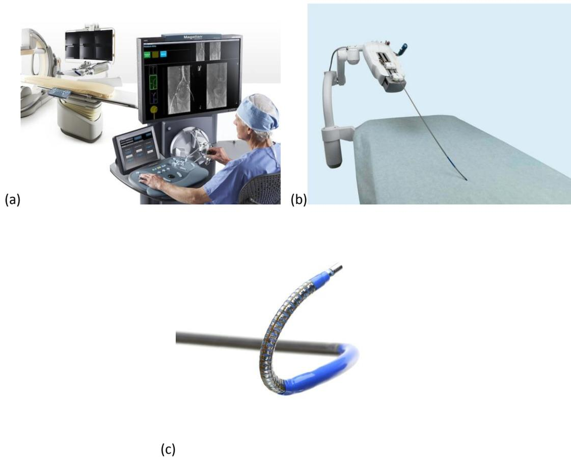
**Figure 11:** Sensei X by Hansen Medical: (a) surgical console; (b) surgical robotic arm (3) Artisan Catheter
