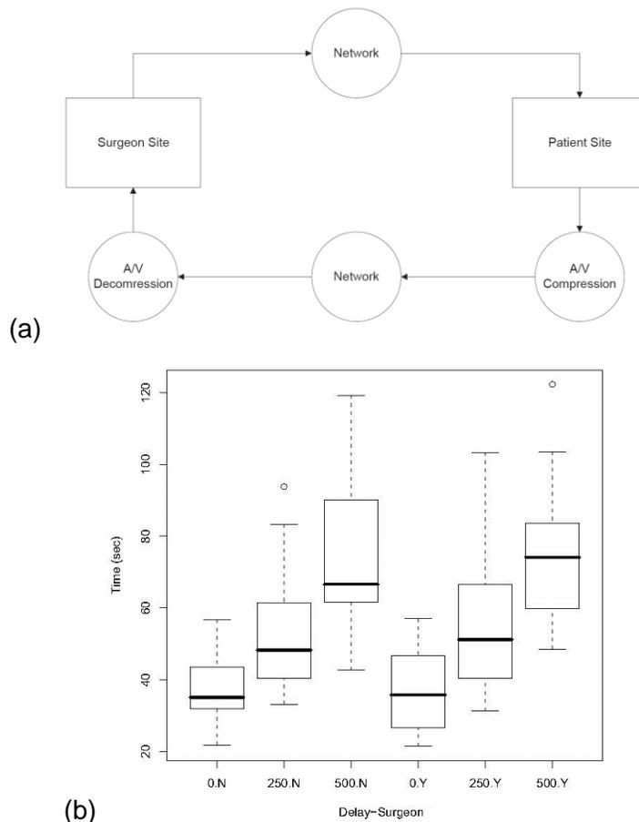
**Figure 7:** Time delay and its effects on surgical performance in telesurgery. (a) Schematic block diagram representing all time delay sources. (b) Completion time of an FLS block transfer as a function of time delay (0, 0.25, 0.5 sec) for surgeons (Y) and non-surgeons (N) using the Raven surgical robotics system in a teleportation mode.
