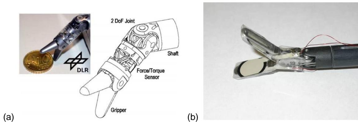
**Figure 6:** Force sensor mounted on the proximal end of a surgical tool (a) DLR endoscopic tool instrumented with a six axis force-torque sensor (b) UCLA Tactile sensor mounted on the faces of a robotic endoscopic grasper.
