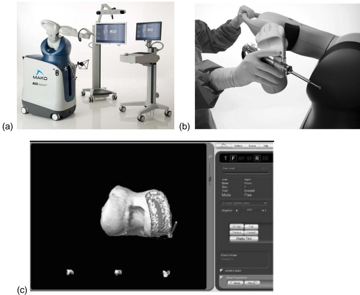
**Figure 12:** Robotic Arm Interactive Orthopedic System (RIO) by MAKO: (a) Overview of the entire system; (b) Shared control of the surgical tool – the surgical robotic arm and the surgeon holding the surgical tool together; (c) Screenshot of the RIO system software showing the model of the patient's femur bone with the planned resection volume
