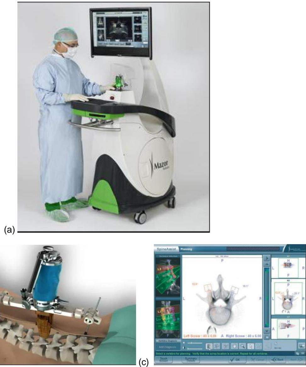
**Figure 14:** (a) Overview of the Renaissance; (b) Mounting Renaissance to the spine; (c) 3D planning of pedicle screws to be introduced into L3 vertebra.
