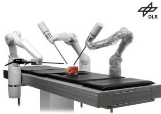
Figure 44.1 The DLR Miro surgical telerobot features three seven degrees of freedom arms with both teleoperation and direct human manipulation capabilities. Image copyright Deutsches Zentrum für Luft- und Raumfahrt, used with permission.
