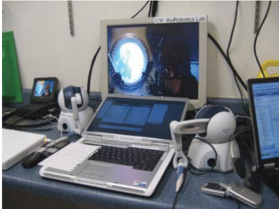
Figure 44.6 RAVEN surgical control site for the NEEMO mission (Figure 44.5). The user interface consists of two Phantom Omni haptic devices and surgical master communication software running on the laptop.
