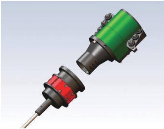
Figure 44.3 Tool interface for the RAVEN I robot can be grasped and exchanged with one hand (either human or robot hand) at the red hexagonal ring.
