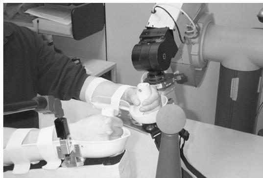
**Fig. 3** Photograph of the MIME robotic system for delivering rehabilitation therapy to patients with arm impairment following stroke. (Photo courtesy of Peter Lum, Virginia Commonwealth University.) (View this art in color at [www.dekker.com](http://www.dekker.com).)
