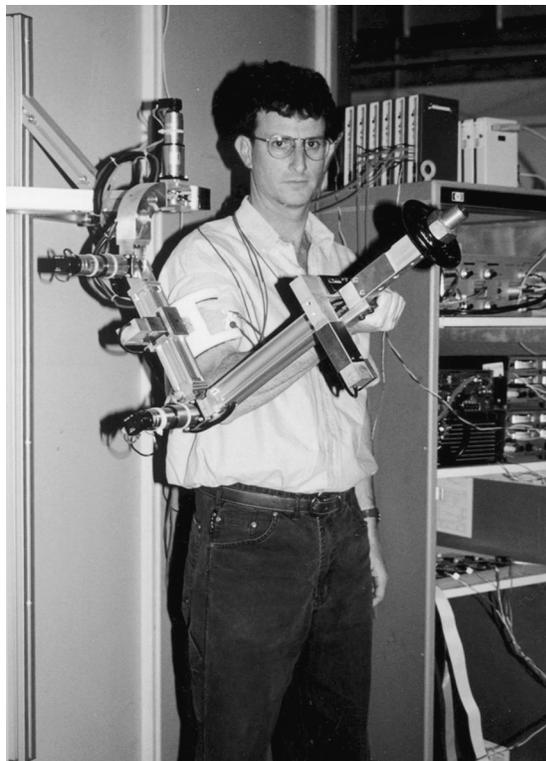
**Fig. 2** Photograph of an exoskeleton for assisting arm movement under development at the University of Washington. (View this art in color at [www.dekker.com](http://www.dekker.com).)
