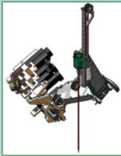
A CAD SHADED IMAGE OF THE SURGICAL ROBOT. CABLE ACTUATED WITH MOTORS ARE MOUNTED ON A STATIC BASE. THE COMPLETE SYSTEM WILL FEATURE TWO MIRROR IMAGE DESIGNED ARMS, ONE FOR EACH OF THE SURGEONS HANDS, PLUS A CAMERA HOLDING/POSITIONING ROBOT.
