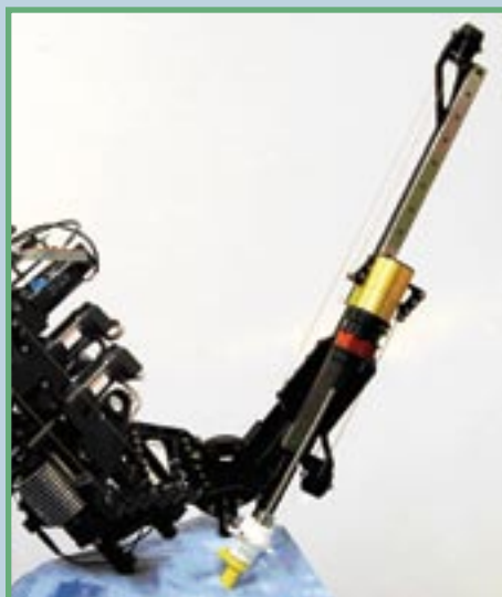
THE BRL 7-DOF SURGICAL MANIPULATOR IS A CABLE-ACTUATED SYSTEM WITH ALL OF THE BRUSHLESS ACTUATORS MOUNTED ON ITS BASE. LINKS WERE OPTIMIZED BASED ON IN-VIVO MIS DATA COLLECTED ON PORINCE MODELS AS WELL AS HUMAN MEASUREMENT. THE COMPLETE SYSTEM INCLUDES TWO ARMS, WITH THE CONTROL SOFTWARE RUNNING ON AN RTAI LINUX COMPUTER.
