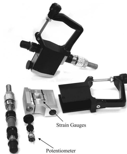
Figure 2. Oarlock sensor, including force and angle transducers.
