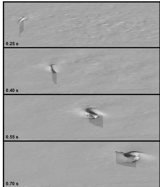
Fig. 9 Evolution of the free surface throughout the stroke. The flow is moving along with the blade sweeping from left-to-right (meaning the shell is moving from right-to-left). Near the end of the stroke there is a surface bulge of approximately 10 cm over and a depression of 8 cm behind the blade
