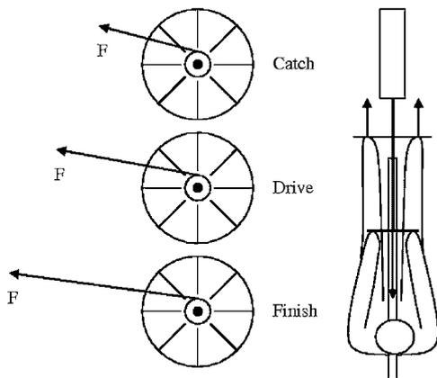
**Figure 2.** Schematic showing system of force transmission from rower to ergometer flywheel.
