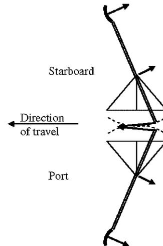
**Figure 3.** Transmission of force from rower to water through the sculls. Dashed lines indicate the movement of the sculls during the stroke.
