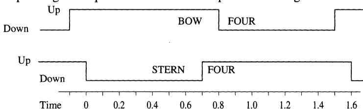
FIGURE 5 Two-phase rowing arrangement for an eight
