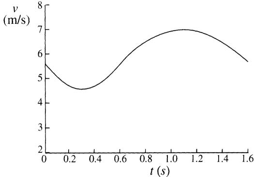
FIGURE 4 Boat velocity  $v$  during one stroke in the 'steady state' situation
