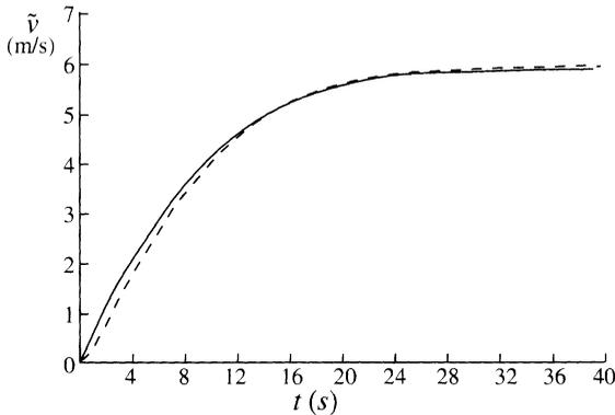
FIGURE 6 Comparison of boat velocity  $\bar{v}$  for single-phase and two-phase rowing during acceleration
