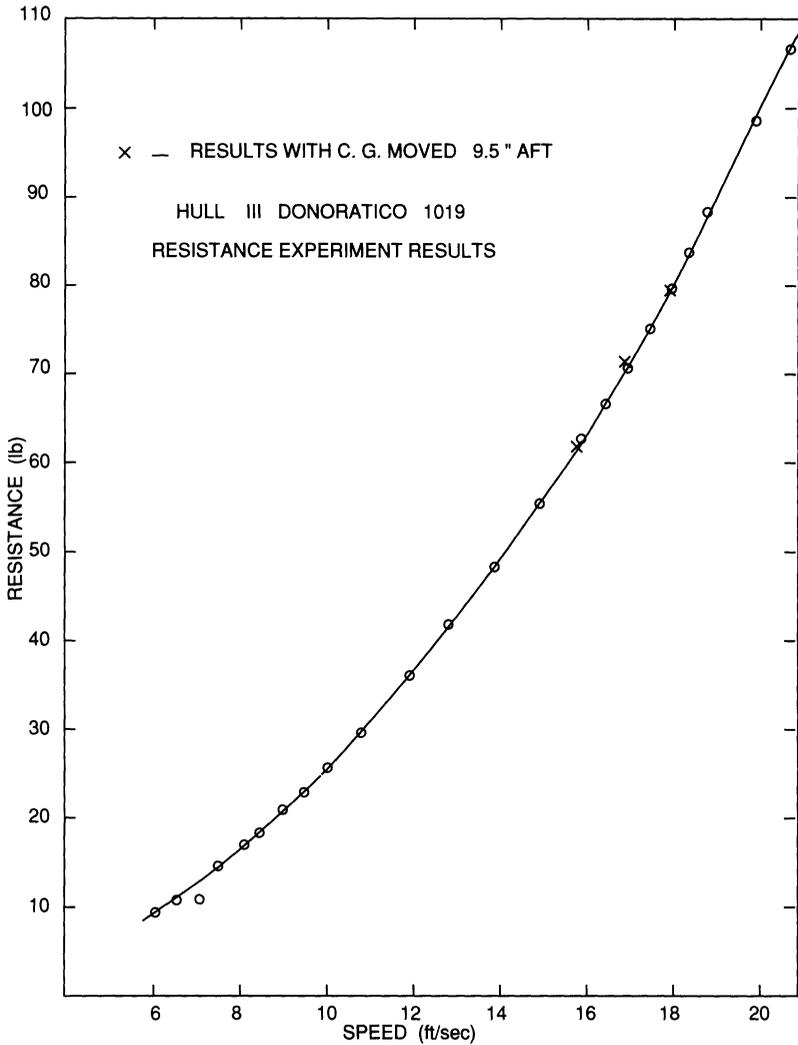
FIGURE 8 Hull resistance in lb wt versus speed in ft/sec for a typical racing eight hull (reproduced from Wellicome (1967) by permission of British Maritime Technology Limited).
