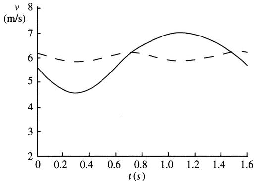
FIGURE 7 Comparison of boat velocity  $v$  for single-phase and two-phase rowing in the 'steady state'
