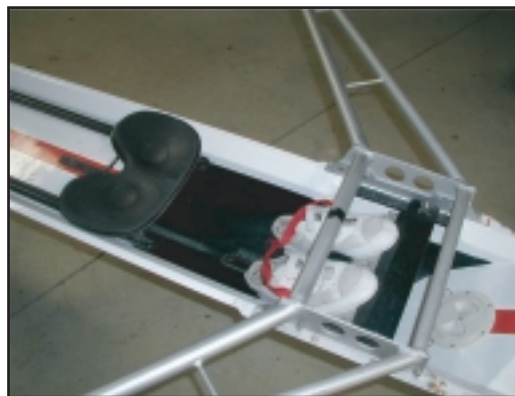
Fig. 1. The inside of a rowing shell. On the left side is the sliding seat on tracks, with the shoes attached to the foot stops on the right. Over the top is the aluminium rigger extending outward from the boat.
