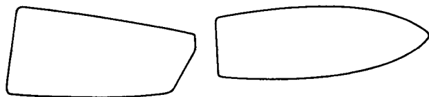
Fig. 2. The new blade introduced in 1991 (left) being rectangular in shape, broader and shorter compared with the traditional blade (right).
