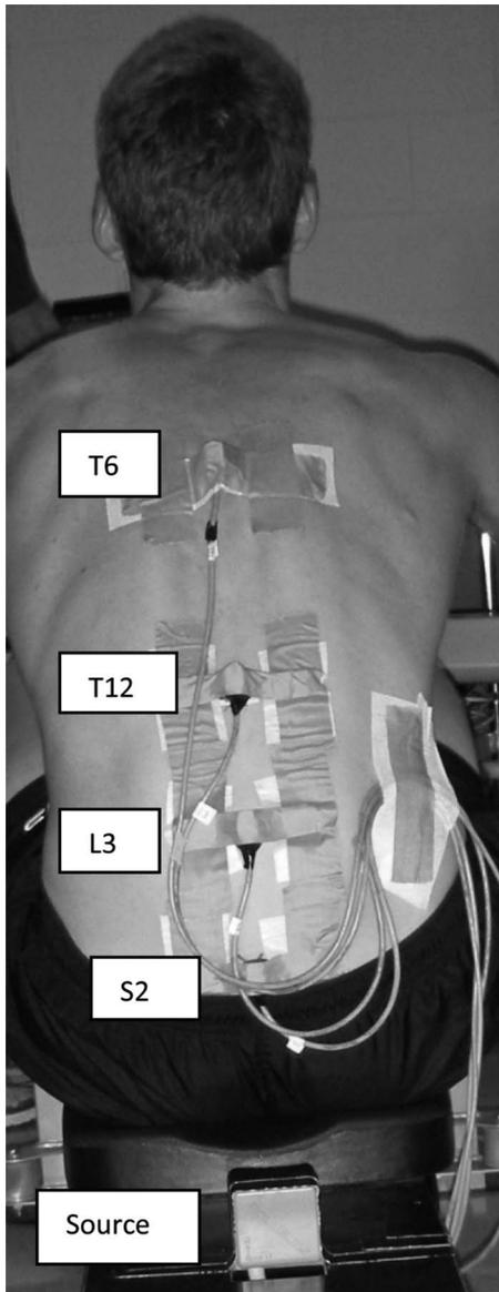
**FIGURE 2.** Placement of the sensors from the 3-Space Fastrak on a rower during testing.
