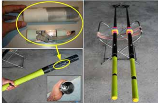
Figure 4. Mounting the mote inside the oar.
