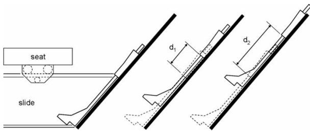
Figure 2. (A) The original Concept 2 foot stretcher position relative to the seat (position 1). (B, C) The two new positions for the foot stretcher, with  $d_1 = 5$  cm (position 2) and  $d_2 = 10$  cm (position 3).
