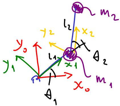
$$\overset{\circ}{1}T = \left[ \begin{array}{ccc|c} c_1 & -s_1 & 0 & 0 \\ s_1 & c_1 & 0 & 0 \\ 0 & 0 & 1 & 0 \\ \hline 0 & 0 & 0 & 1 \end{array} \right]$$
