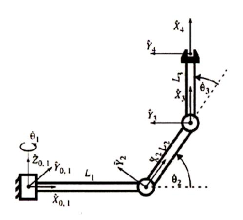
$${}^{4}v_{4} = \begin{bmatrix} L2s3\dot{\theta}_{2} \\ (L2c3 + L3)\dot{\theta}_{2} + L3\dot{\theta}_{3} \\ -(L1 + L2c2 + L3c23)\dot{\theta}_{1} \end{bmatrix}$$
