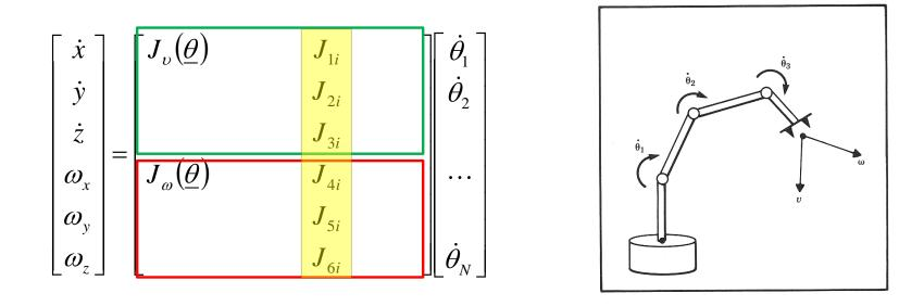
• The i'th column maps the contribution of the angular velocity of the i'th joint to the linear and angular velocities of the end effector along all the axis (x,y,z)
