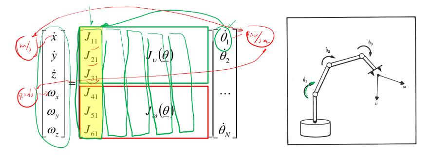
• The first column maps the contribution of the angular velocity of the first joint to the linear and angular velocities of the end effector along all the axis (x,y,z)
