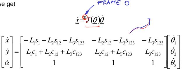
The Jacobian provides a linear transformation, giving a velocity map and a force map for a robot manipulator. For the simple example above, the equations are trivial, but can easily become more complicated with robots that have additional degrees a freedom. Before tackling these problems, consider this brief review of linear algebra.
