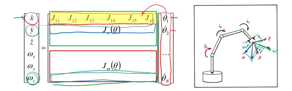
• The first line maps the contribution of the angular velocity of each joint to the linear velocity of the end effector along the x-axis
