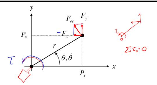
• The moment about the joint generated by the force acting on the end effector is given by
