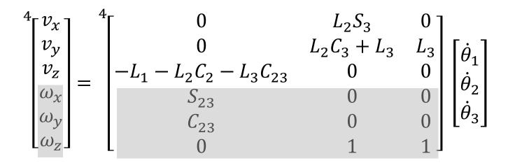
• The resulting reduced Jacobian will be square (the number of independent rows in the Jacobian are equal to the number of unknown variables) and can be inverted unless in a singular configuration.
