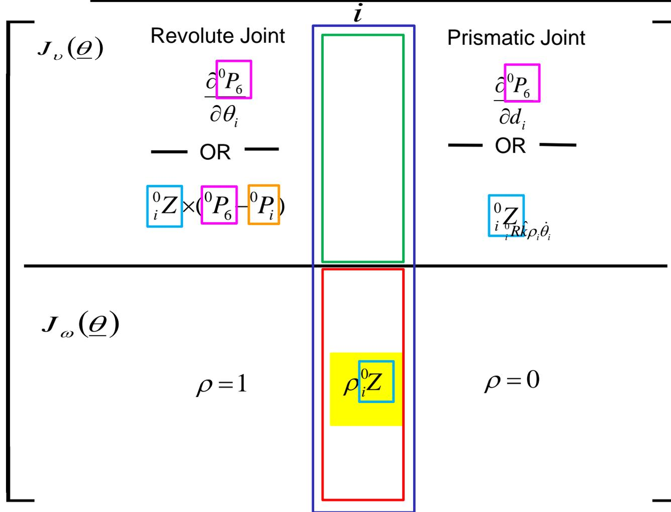
$${}^0T_i = \left[ \begin{array}{ccc|c} * & * & {}^0Z_{ix} & {}^0P_{ix} \\ * & * & {}^0Z_{iy} & {}^0P_{ix} \\ * & * & {}^0Z_{iz} & {}^0P_{ix} \\ \hline 0 & 0 & 0 & 1 \end{array} \right]$$
