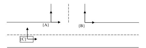
• The velocity of the object in {C} relative to both {A} and {B} is the same, that is
