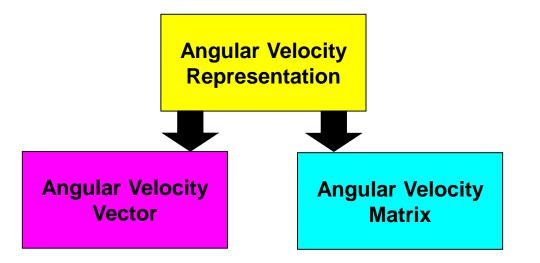
• The angular velocity vector is convenient to use because it has an easy to grasp physical meaning. However, the matrix form is useful when performing algebraic manipulations.
