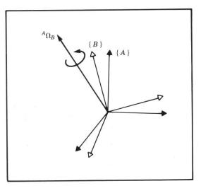
• The angular velocity vector  ${}^{A}\Omega_{B}$  describes the instantaneous change of rotation of frame {B} relative to frame {A}
