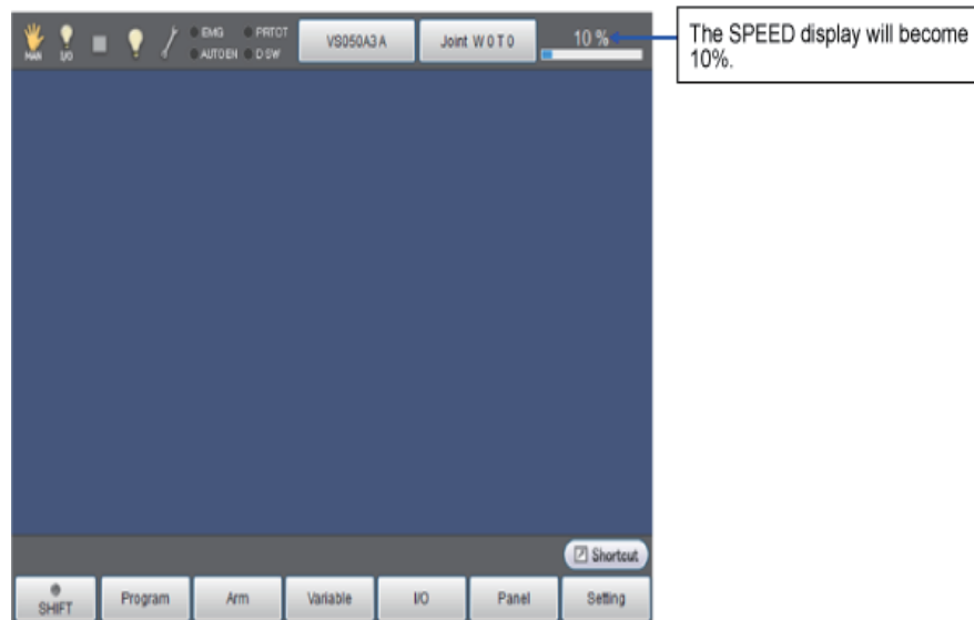
Figure 18: Step 3 of running the robot manually
