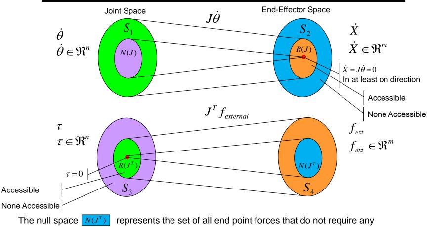
torques at the joints to bear the corresponding load • (e.g. 2R fully stretched or collapsed elbow).
