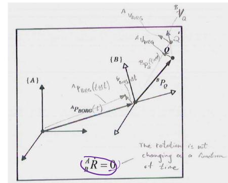
$${}^{A}V_{Q} = {}^{A}V_{BORG} + {}^{A}({}^{B}V_{Q}) = {}^{A}V_{BORG} + {}^{A}_{B}R^{B}V_{Q}$$
