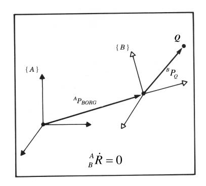
$${}^{A}V_{Q} = {}^{A}V_{BORG} + {}^{A}({}^{B}V_{Q}) = {}^{A}V_{BORG} + {}^{A}_{B}R^{B}V_{Q}$$
