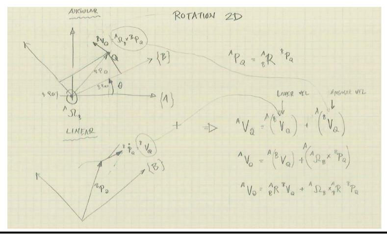
$$AV_{Q} = {}^{A}V_{BORG} + {}^{A}_{B}R^{B}V_{Q} + {}^{A}\Omega_{B} \times {}^{A}_{B}R^{B}P_{Q} \qquad AV_{Q} = {}^{A}V_{BORG} + {}^{A}_{B}R^{B}V_{Q} + {}^{A}_{B}\dot{R}_{\Omega}\left({}^{A}_{B}R^{B}P_{Q}\right)$$
