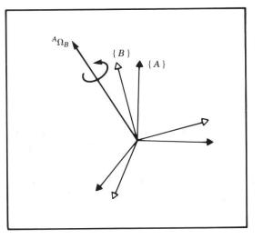
• The angular velocity vector  ${}^{A}\Omega_{B}$  describes the instantaneous change of rotation of frame {B} relative to frame {A}
