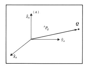
$${}^{A}V_{Q} = \frac{d}{dt} {}^{A}P_{Q} \approx \lim_{\Delta t \to 0} \frac{{}^{A}P_{Q}(t + \Delta t) - {}^{A}P_{Q}(t)}{\Delta t} \approx \lim_{\Delta t \to 0} \frac{{}^{A}P_{Q}(t) - {}^{A}P_{Q}(t - \Delta t)}{\Delta t}$$
