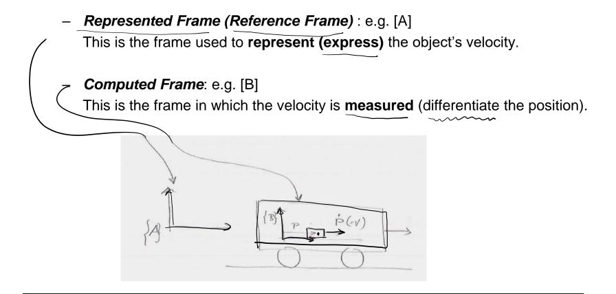
$$= {}^{A}V_{Q} = {}^{A}V_{BORG} + {}^{A}_{B}R^{B}V_{Q} + {}^{A}\Omega_{B} \times {}^{A}_{B}R^{B}P_{Q} \qquad {}^{A}V_{Q} = {}^{A}V_{BORG} + {}^{A}_{B}R^{B}V_{Q} + {}^{A}_{B}\dot{R}_{\Omega}\left({}^{A}_{B}R^{B}P_{Q}\right)$$
