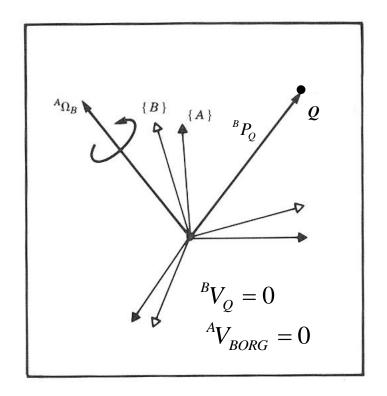
$${}^{A}V_{Q} = {}^{A}V_{BORG} + {}^{A}_{B}R^{B}V_{Q} + {}^{A}\Omega_{B} \times {}^{A}_{B}R^{B}P_{Q} \qquad {}^{A}V_{Q} = {}^{A}V_{BORG} + {}^{A}_{B}R^{B}V_{Q} + {}^{A}_{B}\dot{R}_{\Omega} \left( {}^{A}_{B}R^{B}P_{Q} \right)$$
