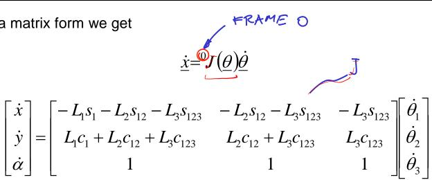
The Jacobian provides a linear transformation, giving a velocity map and a force ٠ map for a robot manipulator. For the simple example above, the equations are trivial, but can easily become more complicated with robots that have additional degrees a freedom. Before tackling these problems, consider this brief review of linear algebra.
