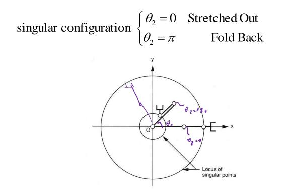
• The manipulator loses 1 DEF. The end effector can only move along the tangent direction of the arm. Motion along the radial direction is not possible.
