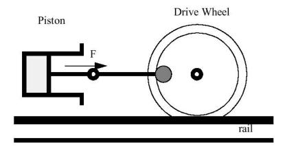
• The piston force, F, cannot generate any torque around the drive wheel axis because the linkage is singular in the position shown.
