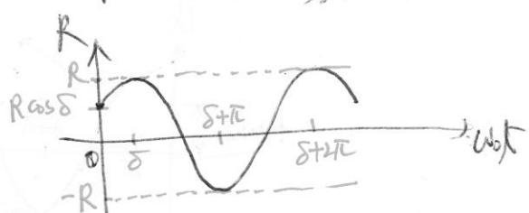
$$\text{period: } T = \frac{2\pi}{\omega_0} = 2\pi \left( \frac{m}{k} \right)^{\frac{1}{2}}, \omega_0 = \text{natural freq.}$$
