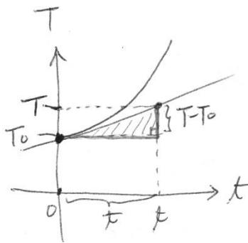
$$\frac{T - T_0}{t - 0} = \left. \frac{dT}{dt} \right|_{t=0} = k(T_0 - T_m)$$
