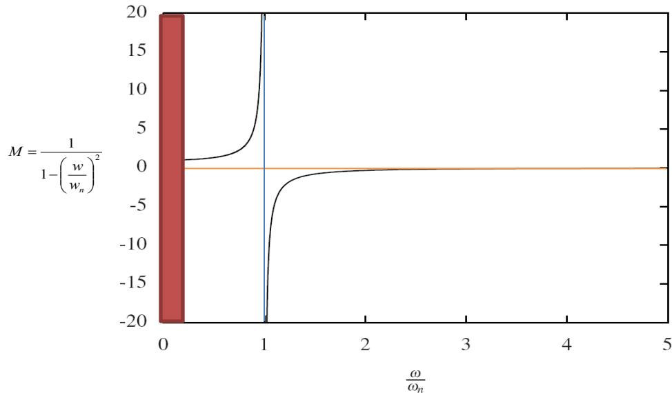
(\*) For  $x(0) = 0, \dot{x}(0) = 0$  and  $\omega \ll \omega_n$   $\left(\frac{\omega}{\omega_n}\right) \rightarrow 0$
