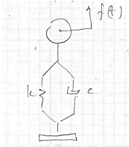
$$m\ddot{x} + cx + kx = f(t) \quad \text{I.C.} \quad \begin{cases} x(t=0) = x_0 = d \\ \dot{x}(t=0) = \dot{x}_0 = v \end{cases}$$
