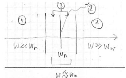
Undamped oscillator  $\zeta = 0 \quad w \neq w_n$  (Case 1)
