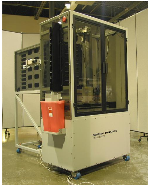
Fig 1 Supply Dispensing Cabinet
